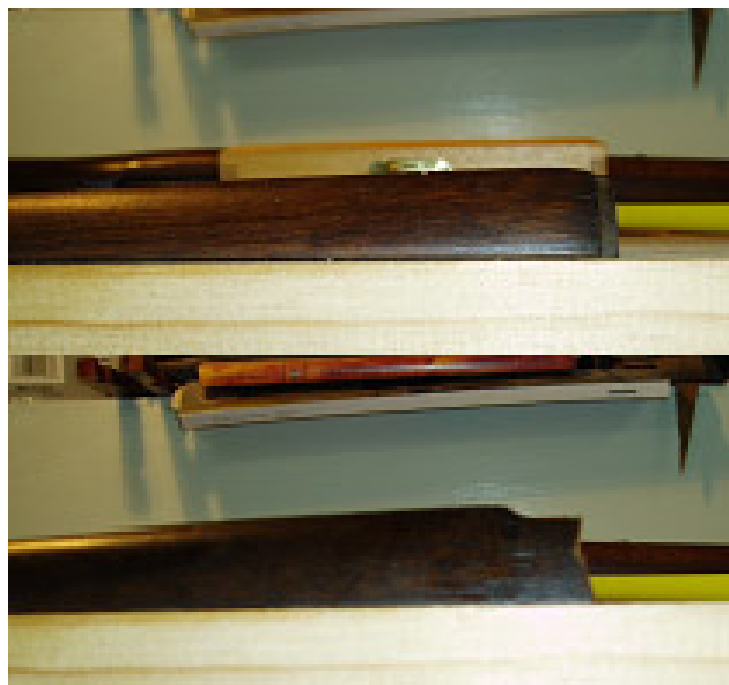
Fig. 11. The original hand guard profile (top) and the initial Cz98/22 profile (bottom)
