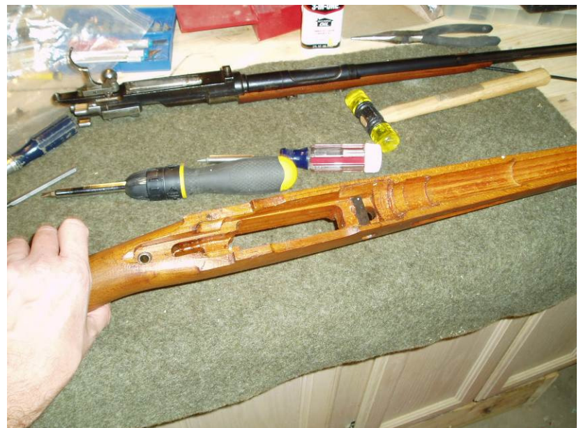
Fig 2. Barrel removed from stock and the upper hand guard ready to be removed and the spring on the rear of the hand guard.
