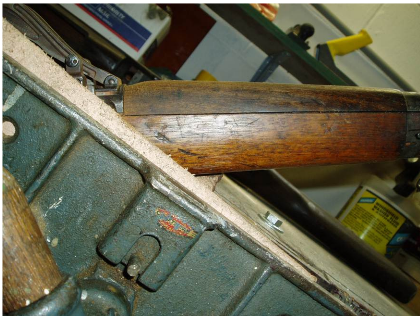
Fig. 15. Profile of guard after sanding. The angle of the 'slope' in front of the Lange sight is slightly more radical than the original.
