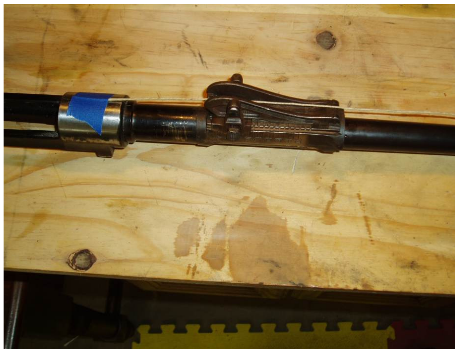
Fig. 7. Aligning the new sight
