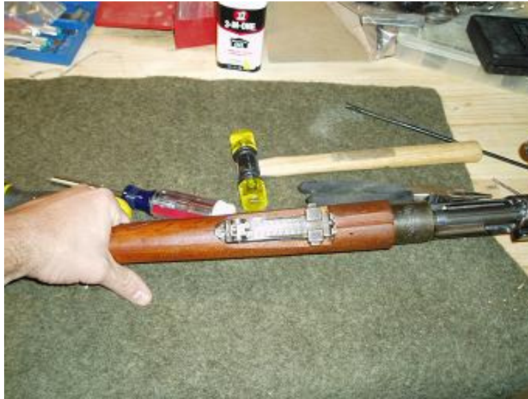
Fig 2. Barrel removed from stock and the upper hand guard ready to be removed and the spring on the rear of the hand guard.
