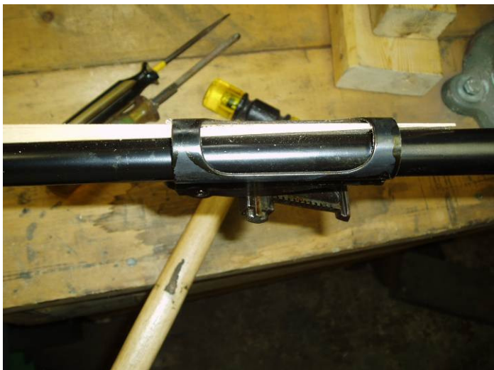
Fig 4 Sight shimmed to protect barrel
