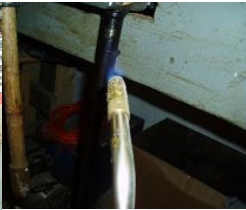
Fig 3. Using a propane torch, the barrel and sight are heated to loosen the solder. Be sure to heat the barrel evenly (above and below the sight) to prevent warping.
