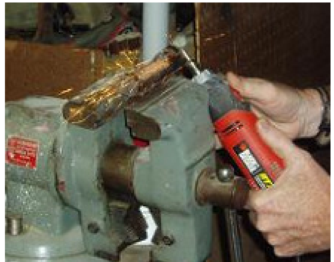
Fig. 5 (Above) Using a dremel fitted with a cutting disk, the bottom of the band is cut, allowing the band to be removed.
