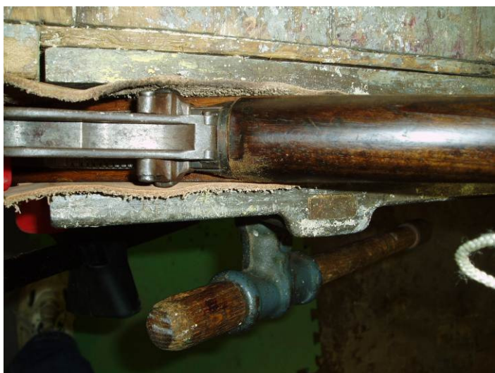
Fig. 14. Shoulders after sanding. Notice the dark spot in the center (the 'dip' from the original guard).
